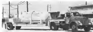
LIQUID fluorine is transferred under pressure of helium gas in the tank truck.
